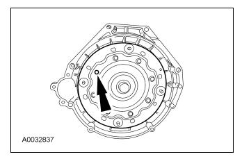
119. Using one of the speed sensor holes, fill the transmission with 8.5L (9 quarts) of automatic transmission fluid.
